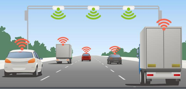
V2X allows vehicles to communicate with other vehicles within the traffic system as well as the infrastructure around them for road safety
